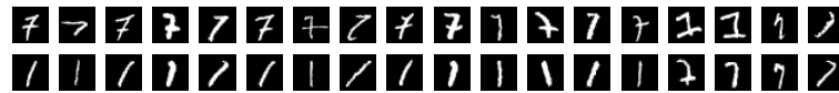
Figure 2.7: The Nearest Neighbour method makes 18 errors out of the 600 test examples. The 18 test examples that are incorrectly classified are plotted (above), along with their nearest neighbour in the training set (below).
