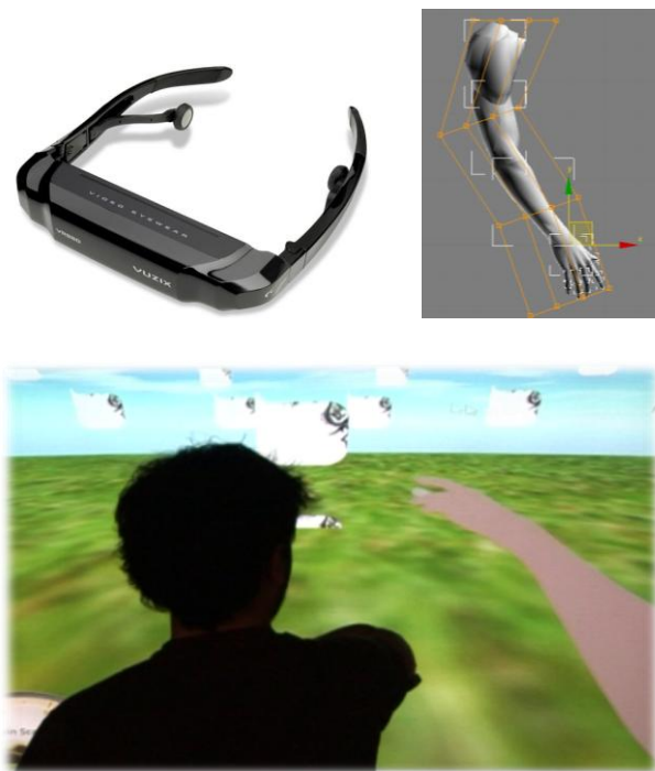
Figure 6. The AR Vuzix iWear VR920 glasses (left-up), the hand model used (right-up) and an amputee user interacting with the Epione Vault via AR-reconstructed hand (down).
