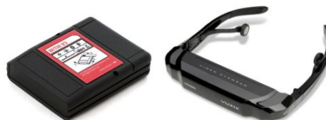
Fig. 5. The hand model used (up), the Wireless accelerometer Sparkfun Witilt v3.0 (down-left), and the AR Vuzix iWear VR920 glasses (down-right).
