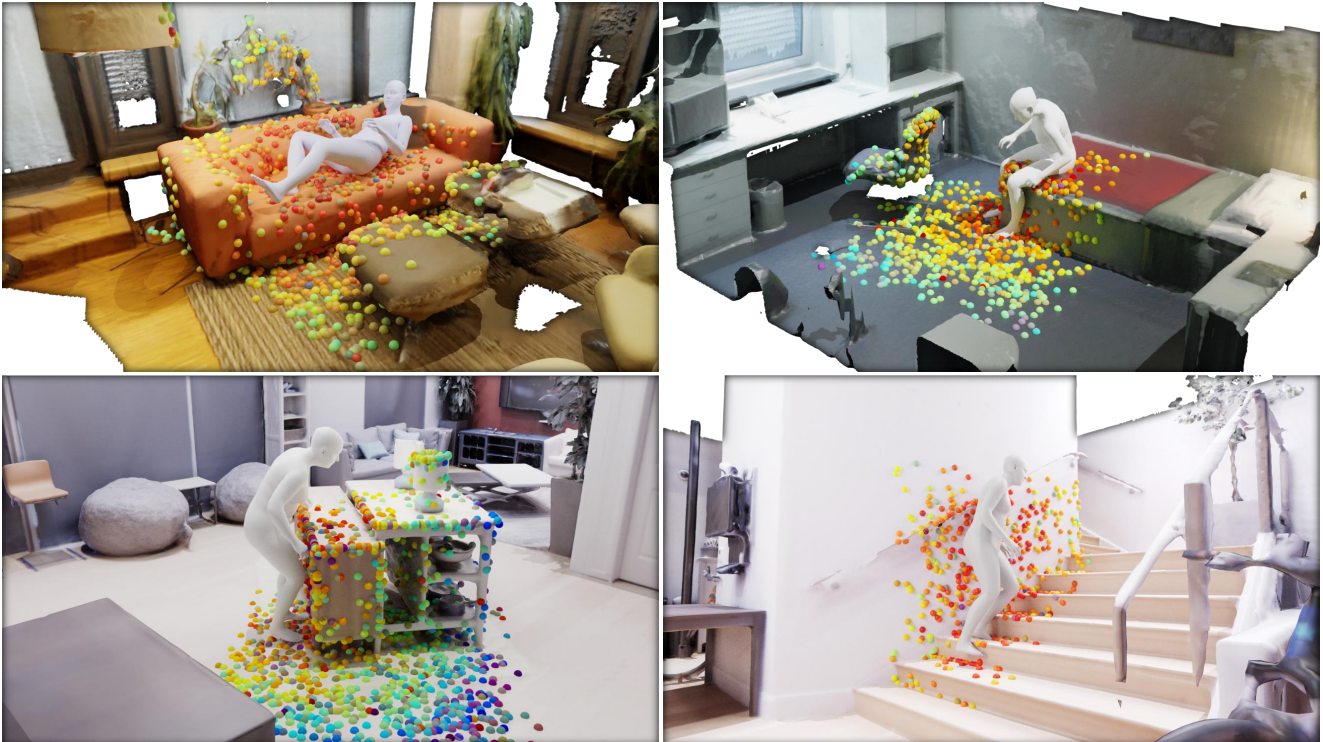
Figure 1: Given a 3D scene mesh, PLACE generates human-scene proximal relationships and infers a plausible human body. The selected local scene vertices are denoted by spheres, and the color denotes the generated minimum distance to the body surface. Distances are normalized to [0, 1] for visualization, and red to purple means close to far.
