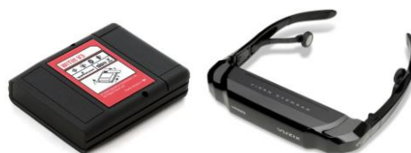
Fig. 5. The hand model used (up), the Wireless accelerometer Sparkfun Witilt v3.0 (down-left), and the AR Vuzix iWear VR920 glasses (down-right).
