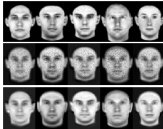
Figure 3: Reconstruction results using subspaces constructed from noisy training data. Top : Original, noiseless, test images. Middle : Least-squares reconstruction of images with standard PCA basis (MSRE 19.35). Bottom : Reconstructed images using RPCA basis (MSRE 16.54).
