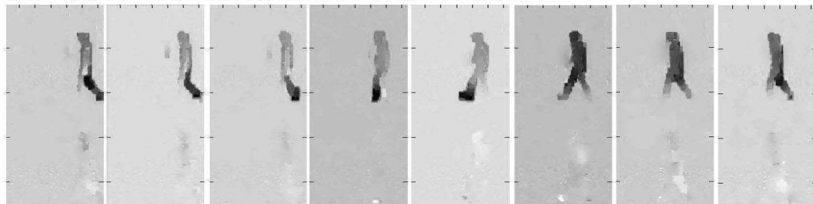
Horizontal (top) and vertical (bottom) components of flow field computed by Black&Anandan's publicly available code.
