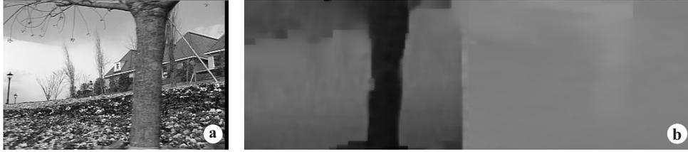
Figure 7. Optical flow estimation: Flower garden sequence. (a) Frame 1 from image sequence. (b) Estimated optical flow with separate  $u$  and  $v$  components.
