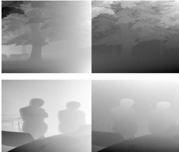
Figure 1. Flow fields generated for an outdoor (top) and an indoor scene (bottom). The horizontal motion  $u$  is shown on the left, the vertical motion  $v$  on the right; dark/light means negative motion/positive motion (scaled to  $0 \dots 255$  for display).
