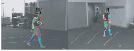
Figure 2: Training Data. Example frames from the training set used to learn human limb likelihoods. The 3D body model is obtained by a commercial motion capture system and is projected into four calibrated camera views. This gives the known position and orientation of the limbs in each view.
