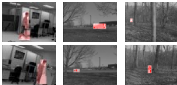
Fig. 1. Detection of moving people (top and bottom) and a moving vehicle (middle) from a hand-carried camera. Each row illustrates two (non-consecutive) frames of long image sequences taken from several seconds apart.
