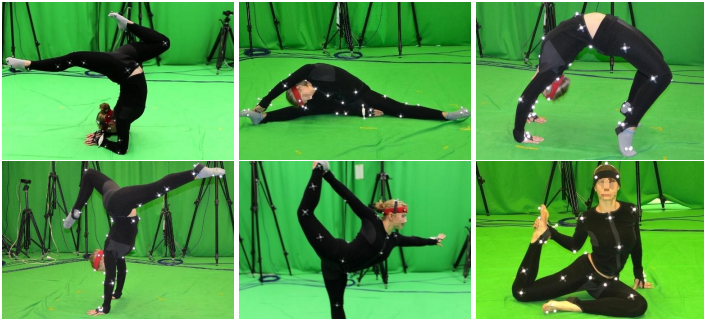
Figure 1: Joint-limit dataset. We captured a new dataset for learning pose-dependent joint angle limits. This includes an extensive variety of stretching poses. A few sample images are shown here. We use this dataset to learn pose-conditioned joint-angle limits. The dataset and the learned joint-angle model will be made publicly available.
